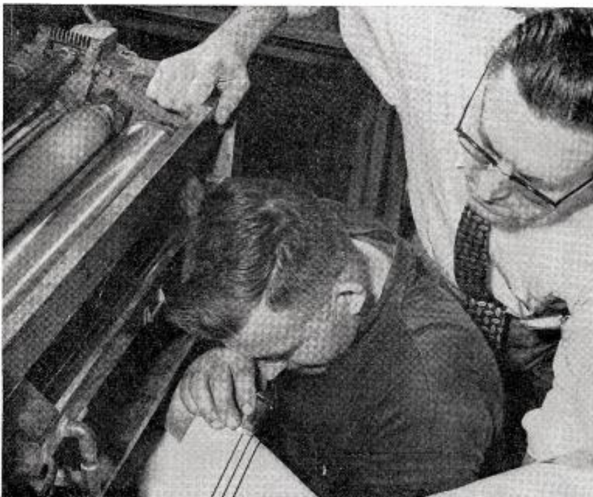
Constant inspection is vital in producing uniform magnetic-ink striping for bank ledgers.
